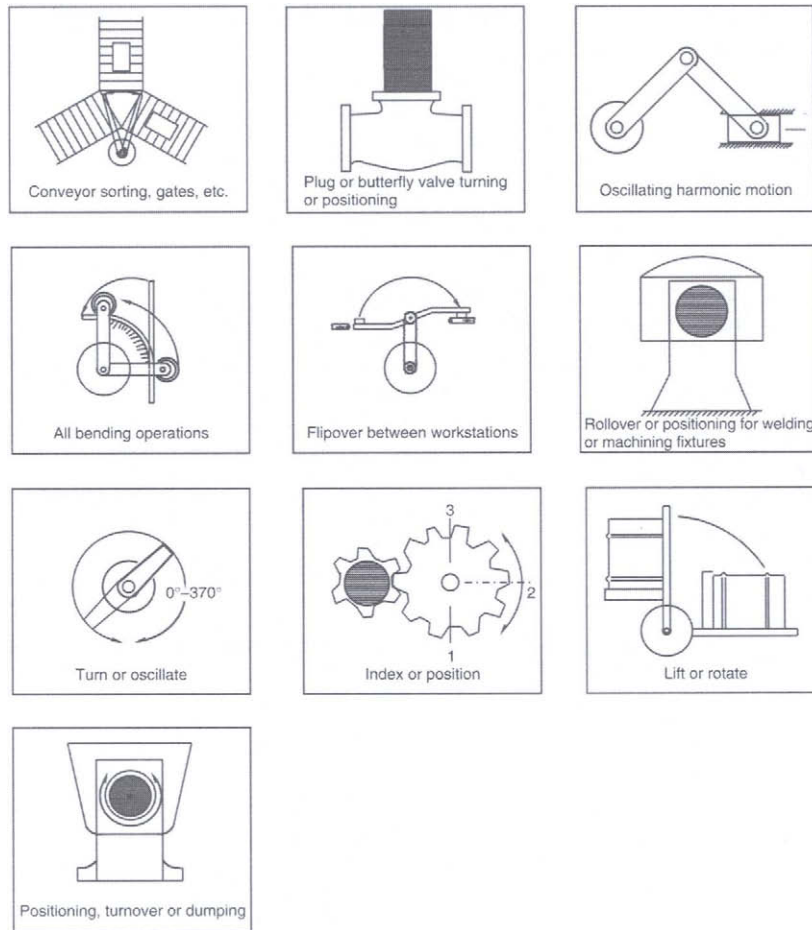
Figure 4.2 Application of limited rotation hydraulic motor
